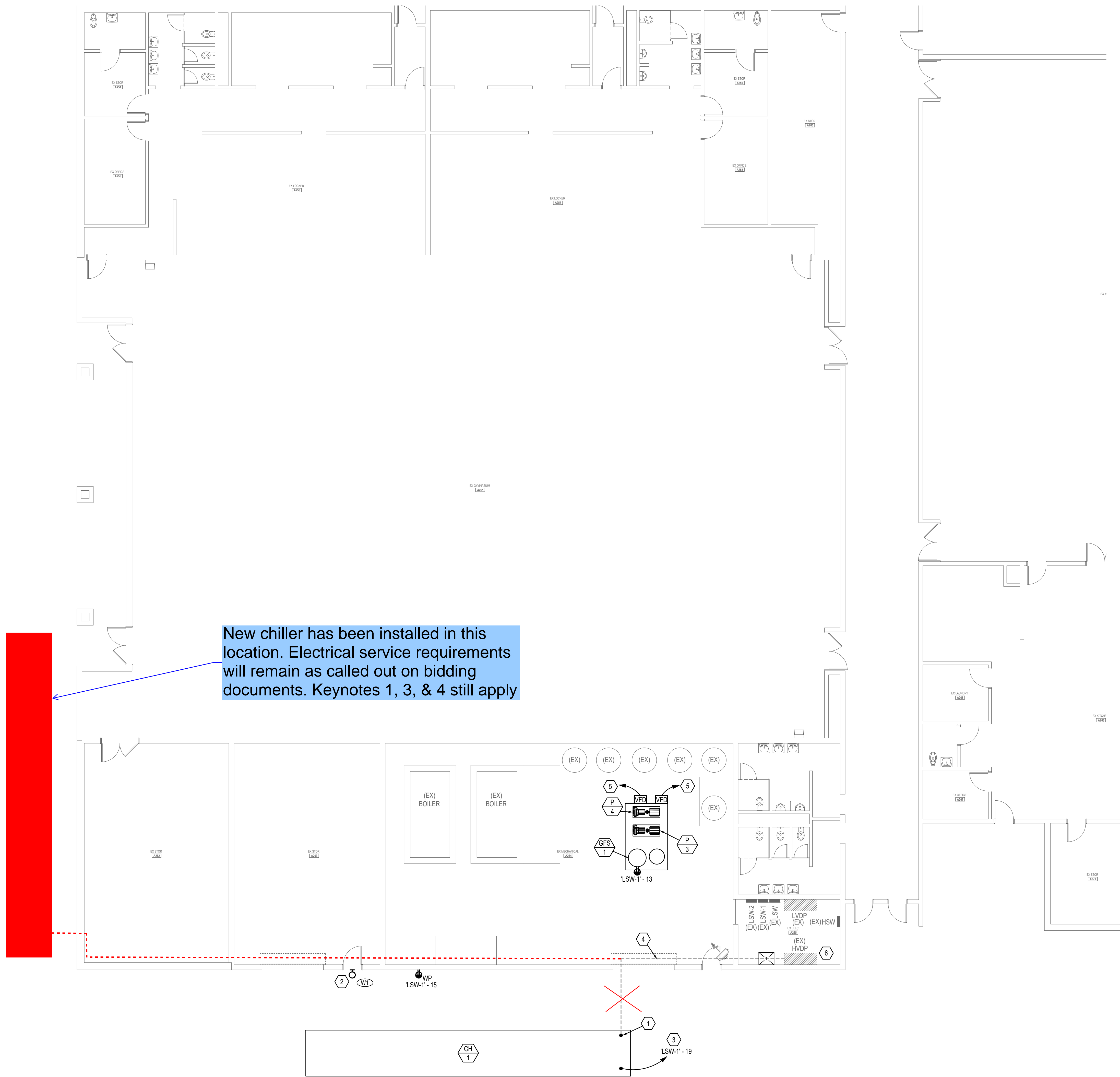
1 AREA 6 - ELECTRICAL PLAN EP1.6 SCALE: 1/8"=1'-0"
